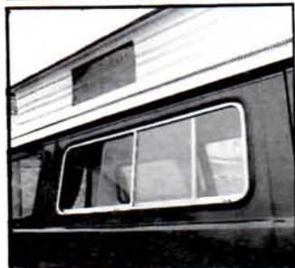
Side windows slide open, extra windows in elevating section
