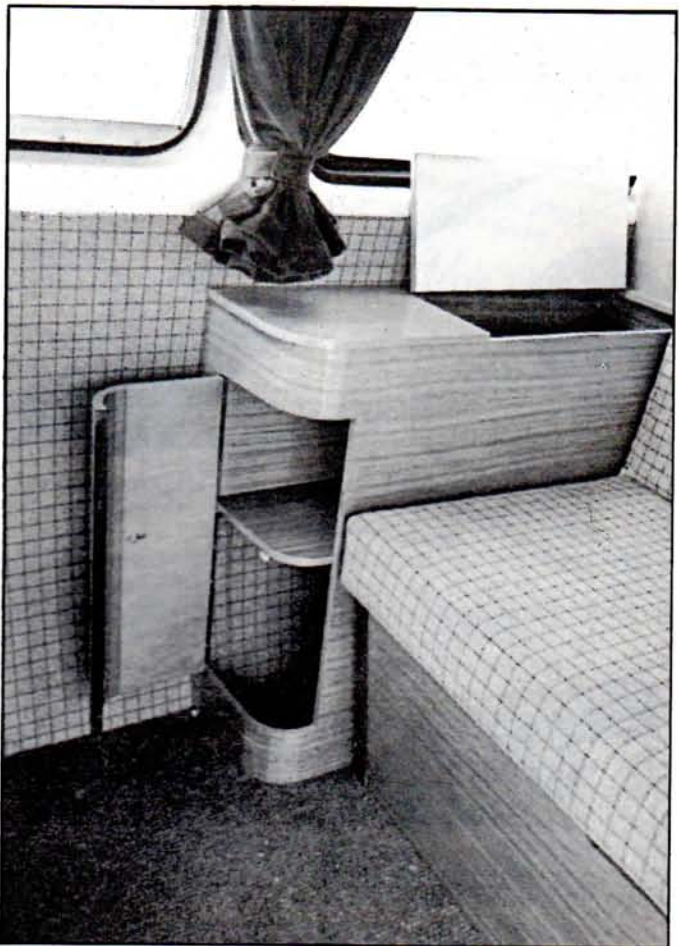
Storage at each side of the van – cupboards and deep lockers
