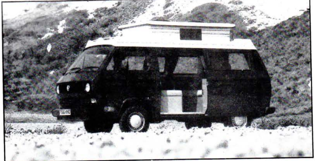
Elevating roof is a simple design which is surprisingly sturdy
