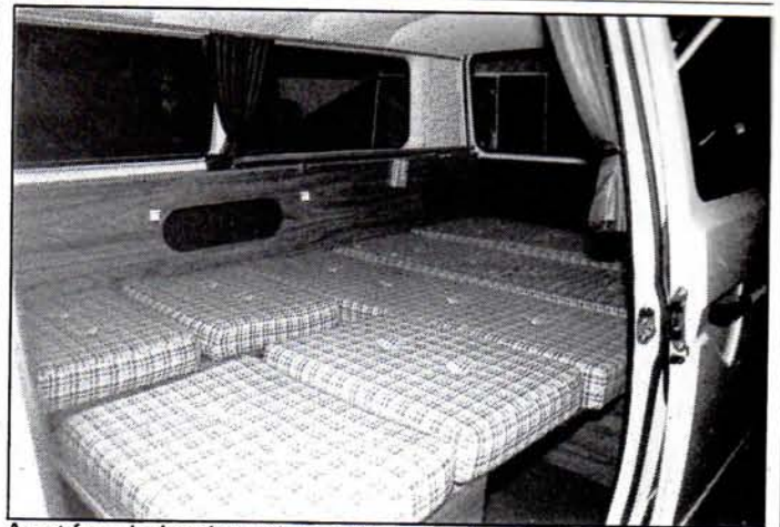
Apart from lockers beneath seats, the only other storage space in the Travellette is in the narrow, full length fitment along the offside wall, where there are pigeon-holes and lids. The enormous bed is made from seat cushions, measures 8ft 2 inches x 4ft 10 inches — but there's a gap at the foot, as shown.
