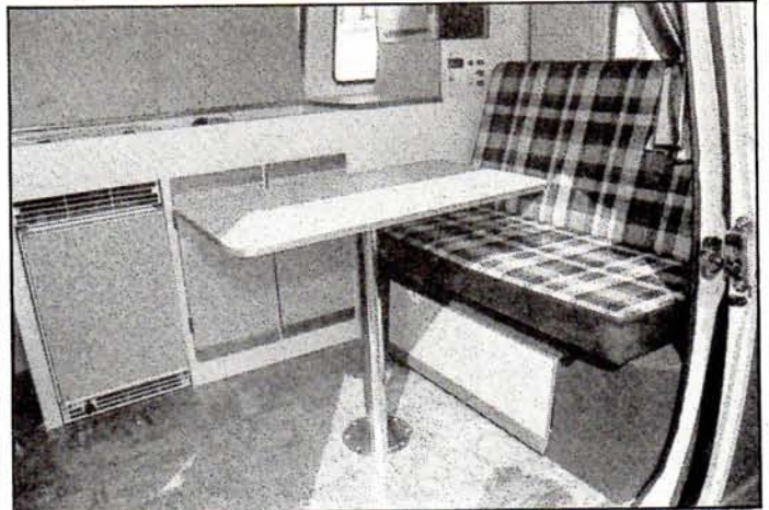
Just as well the table is mounted on a Desmo island leg, so that it can be swivelled to allow the cook to get to the sink and under-sink cupboards. The front of the seat locker is carpeted and the floor is covered with 'cork tile' vinyl.
