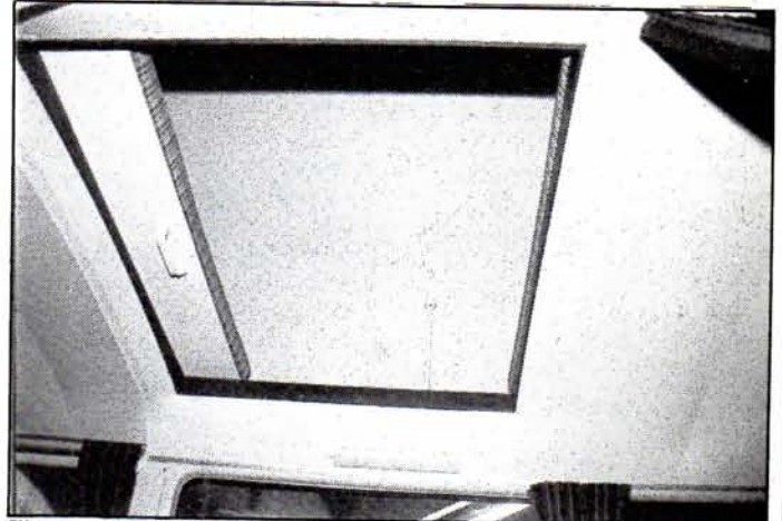
The Travellette's bed in the roof is the same as that on the Series 2, so again it's easier to clamber through the gap shown and then pull the front portion backwards. Travellette is leg generous with interior lighting. There's the one fluorescent shown here, plus two festoons.
