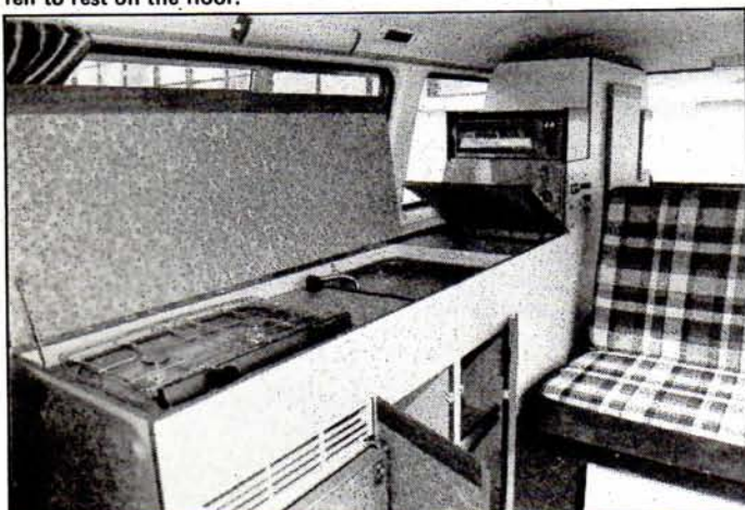
The big lid of the worktop hinges upwards and keeps curtains away from cooking and washing up operations. The commodious top-access locker has its lid partly open. Behind it is the Optimus eye-level grill and, below that, the Zig unit.
