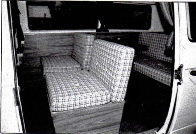
On the Travellette, seven passengers can face forwards for travelling: two in the cab, two on the seats/lockers situated midway and three on the rear bench seat, which is almost five feet wide. There is a narrow gap between the two midway seats.
