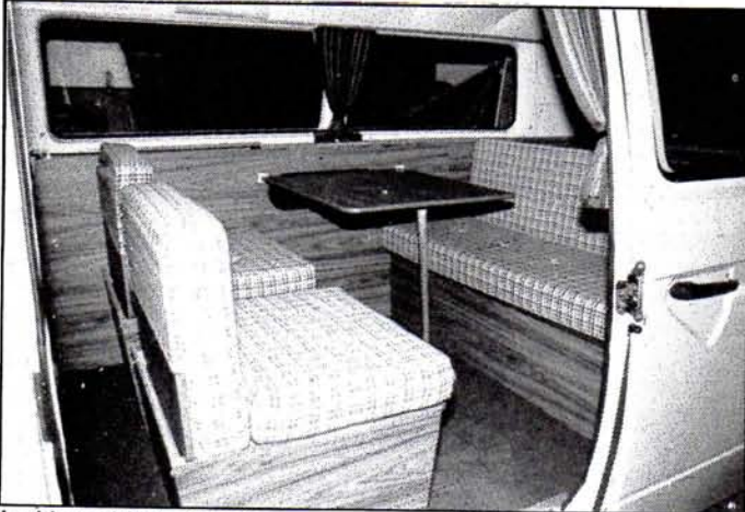
In this model, the two single seats are reversible (though not instantly removable) so that they face the table. Cooker and gas are carried in one of the ventilated underseat lockers. Reversing the seats is simply a matter of pulling out backrests and slotting them in t'other way round.
