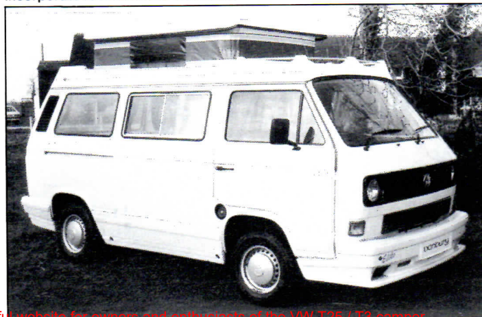
Rising roofs use twin glass fibre shells and have a skirt which folds unaided as the roof is lowered.
