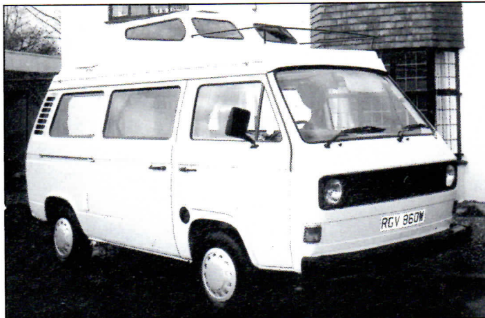
Supervista high tops are cast as a one-piece glass fibre shell and incorporate roof rack and windows.
