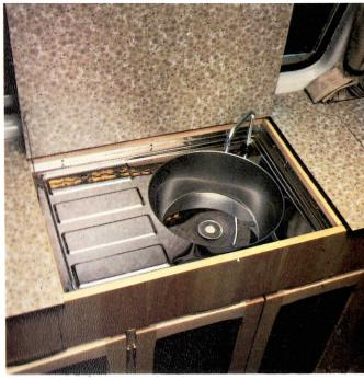
Situated next to the cooker is a beautifully finished stainless steel sink and draining board – large enough for all your requirements, and the 6 gallons of water (contained in  $3 \times 2$  gallon water porters for easy cleaning and maintenance) are fed to the sink by a retractable foot pump.
