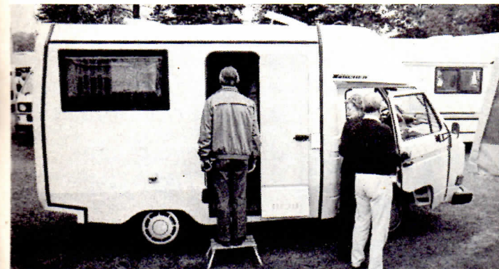
Tischer's 'XN65' on the Transporter, a semi-integrated coachbuilt, which blends the cab into a sandwich-construction body of exceptional strength.
