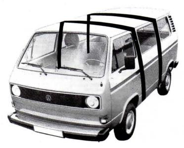
To begin with, there are two strengthening ribs in the roof panel which are welded to vertical pillars; if these are cut or removed the strength of the body shell and the safety of passengers will be impaired.
